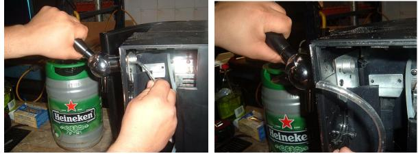
4.) Next, insert the new hose the same way you removed the old one. Pull and hold the lever down and insert the new hose from the back. Keep pushing the hose in until you can see it coming out the faucet. Then pull it back about 1/4 inch. Reattach the hose to the beer line and then screw on the coupler as pictured below and your done. Then put the side panel back on.
